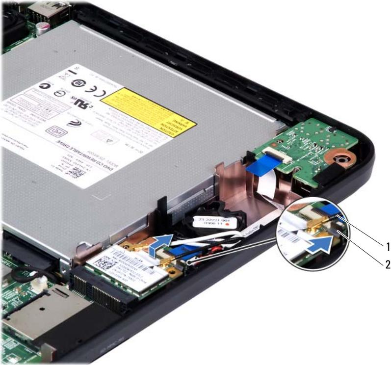
1 kabel antena Mini-Card (2)
